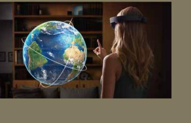
The Microsoft Hololens, revealed in early 2015 and released in 2016, brings mixed reality and spatial computing into one head-mounted display. The Hololens display projects light through flat, transparent optical waveguides that are matched to an environment pre-scanned by a system of cameras. Using the Hololens to display information can allow datasets to be present in a three-dimensional space alongside real-world, on-screen datasets for decision making.
